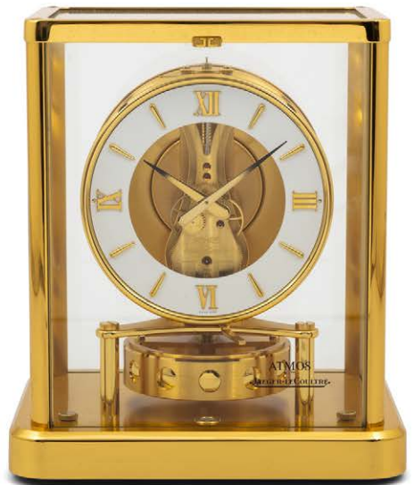
Jaeger-LeCoultre atmos clock in a polished gold plate finish. With atmospheric movement that does not require winding. Switzerland, Circa 1970
